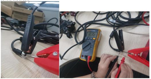
Above picture are use 12V of bench to simiulate car battery, black clip connect with negative electrode '-', read with positive electrode '+'.
