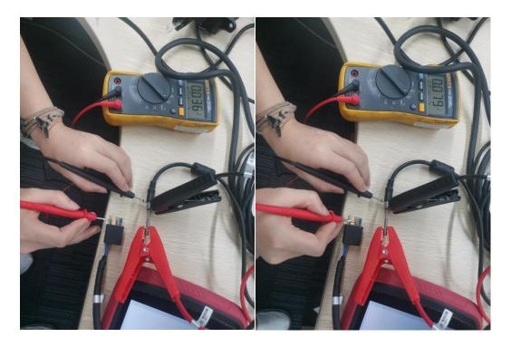
Then try test two pins again after turn on the voltage.(normal situation is output 12V)
