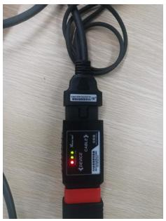
You need to ensure three light are on, if connection is no problem but lights not on, try re-plug the J6 plug.
